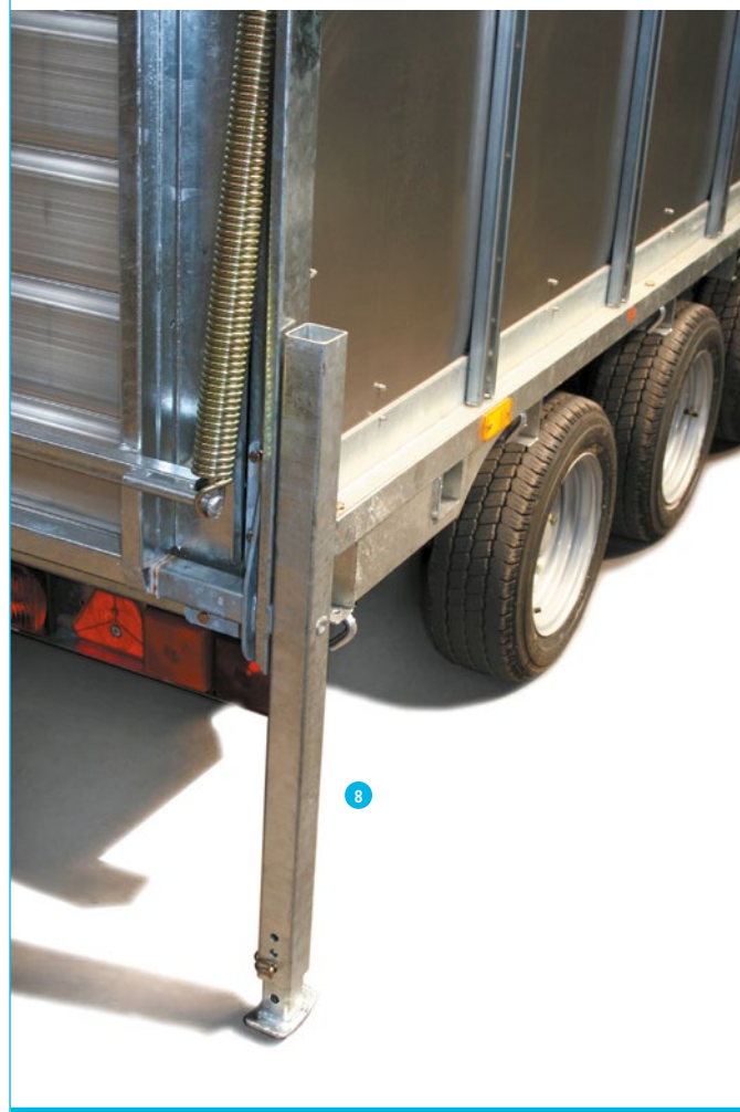
8 KX4950 DP Container Removal Kit. Includes 4 adjustable legs, adjustment tool, fittings & guide to remove and refit the DP container. For fitting to Tri-axle trailers please contact our technical department for guidance prior to purchase.
